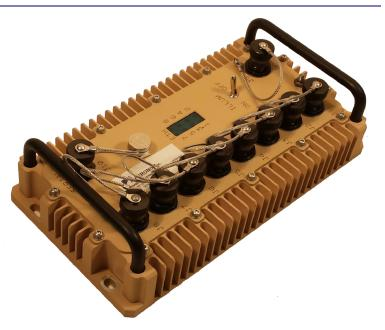
The Aeronix Gigabit Ethernet Switch (GES) GV8m provides eight Tri-speed 10/100/1000 BASE-T Ethernet ports for use in commercial, industrial, and military applications that require ultra-high data transfer rates in a self contained ruggedized package. The GV8m was designed for Ground Vehicle applications that require a rugged package with individual interface connectors. The GV8m meets rigorous environmental, EMI and EMC requirements specifically to meet Ground applications.
