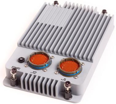
The Aeronix Gigabit Ethernet Switch (GES) Gen2 provides twelve Tri-speed Ethernet ports for use in commercial, industrial, and military applications that require ultra-high data transfer rates in a self contained ruggedized package. The rugged design requires no forced air or conductive cooling, allowing operation in a broad range of harsh environments including operation in uninhabited aircraft bays.
