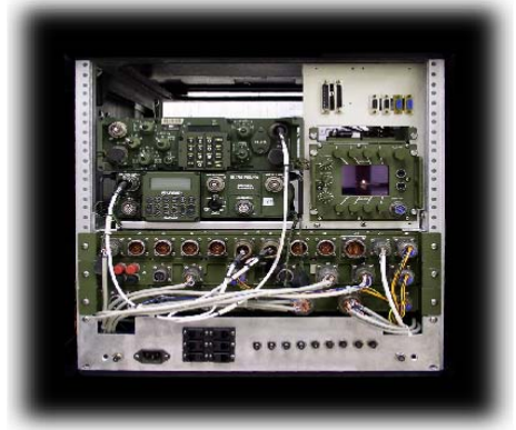
UCIM Rack Mounted Components Installed in Standard Rack for Easy Deployment
